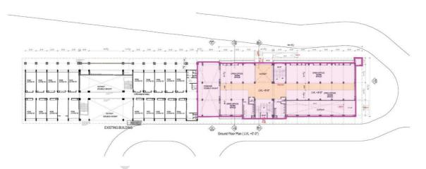
Image 25: Proposed Plan of Block-3 with red indicating the modification/extension to the existing building; Green indicates the new block Ground Floor © Satnam Namita and Associates
